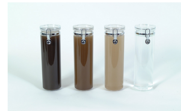
Water samples from the EnwaMatic® technology. Day 1 to day 30 from left to right.
